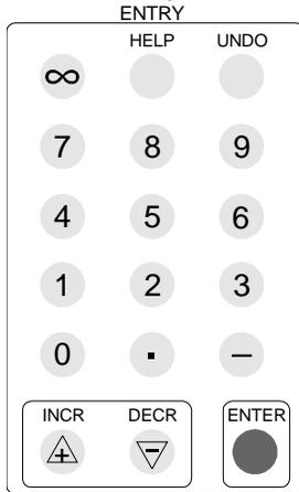
The ENTRY section of the keypad is used to navigate around the 3800 keyboard and make parameter entries into the display fields.
