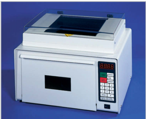
Translinker features a UV crosslinker and transilluminator.
