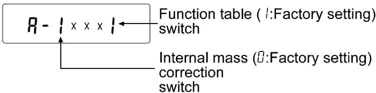
Set the function table switch and internal mass correction switch to “1” as shown above using the following keys.
