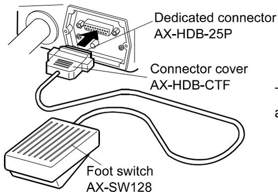
The external input connector (AX-HDB-25P/CTF) and the foot switch (AX-SW128) are sold separately.
