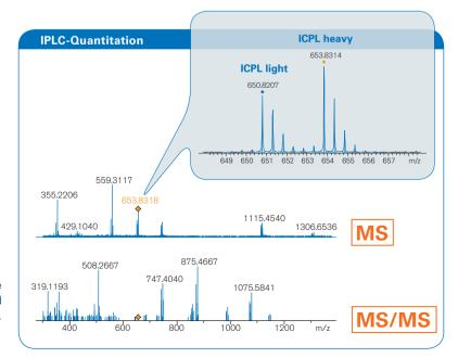
ICPL quantitation on the micrOTOF-Q in MS and MS/MS mode.
