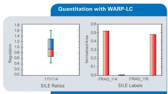
WARP-LC quantitation analysis: Box-and-whisker plot of an iTRAQ labeled protein. For validation, the statistical distribution is shown.
