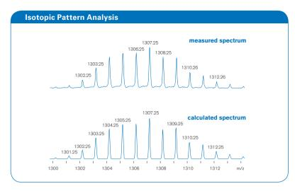
MS analysis of Pd-Complex ( $C_{61}H_{65}N_4O_{15}$ ) in synthetic chemistry. Isotopic Pattern of measured spectrum and calculated spectrum (SigmaFit) show outstanding homogeneity, providing a superior sigma value for enhanced confidence in structural analysis.
