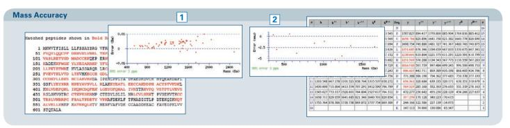
Reproducible mass accuracy: 50 fmol BSA on a Waters UPLC™ column are measured with an RMS error of only 2ppm (1). Even fragments are reliably analyzed (2) with only 3 ppm RMS error (20 fmol BSA) from a single external calibration.
