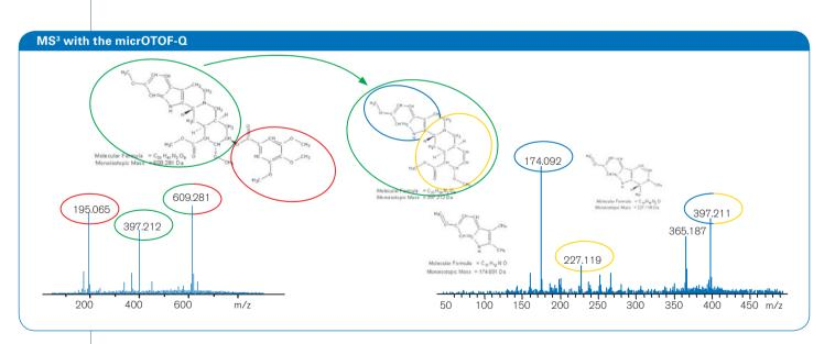
Reserpine: In-Source CID, Isolation of ISCID ions and fragmentation: MS<sup>3</sup>.
