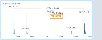
Distinction of sulfation and phosphorylation with micrOTOF-O's accurate mass measurement capabilities.
